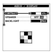
backlight, highlight the "Backlight" label, then use the left and right arrow keys to change the light's intensity.
